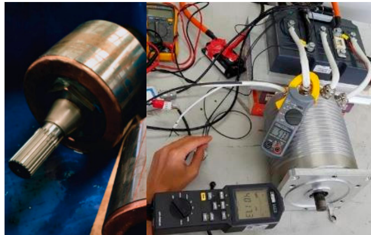
Figure 9. Copper rotor and E-engine prototype at no-load testing at 4017 rpm.
