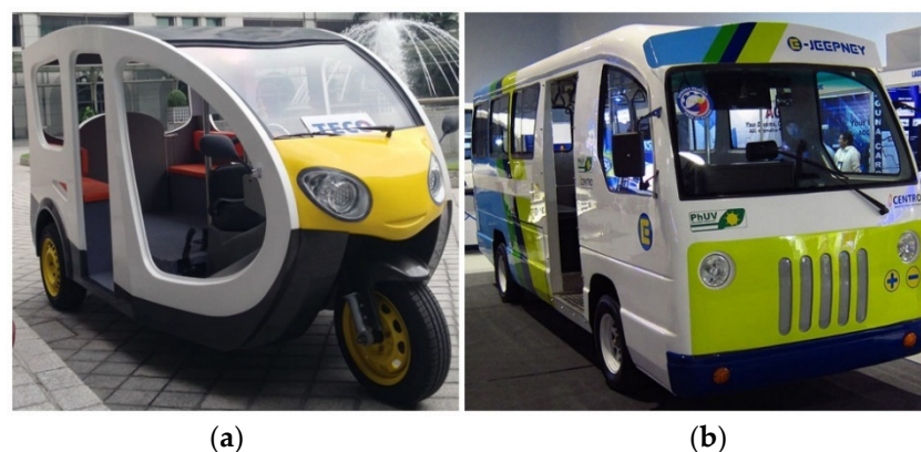
Figure 1. Modernized public utility vehicles (PUVs) in the Philippines: (a) e-trike and (b) e-jeepney. Source: Top Gear Philippines.
