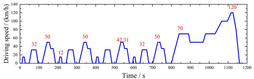
**Figure 2.** NEDC working condition curve.
