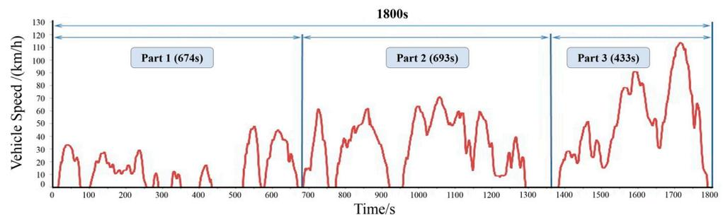
**Figure 3.** CLTC-P working condition curve.
