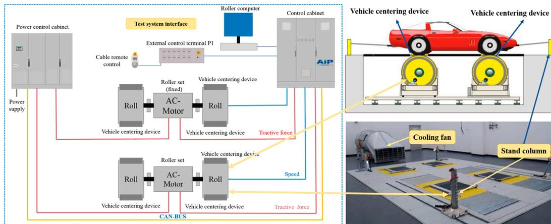
**Figure 4.** The diagram of the test device and interface.
