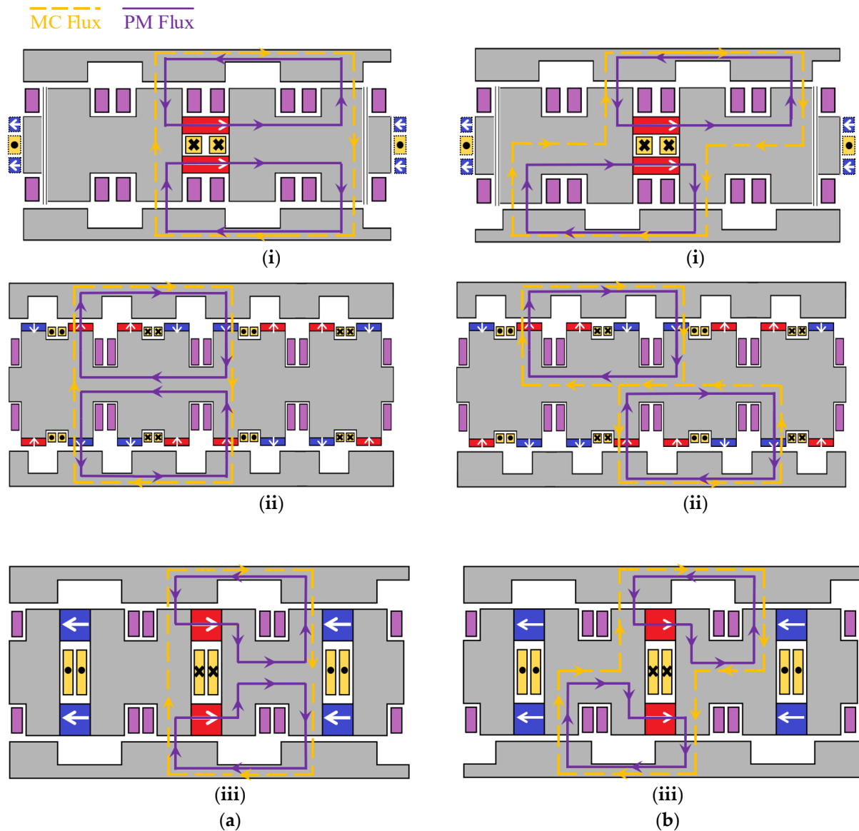
Figure 2. Operation principles of three AF-DR motors with rotors. (a) Aligned position: (i) DSPM, (ii) FRPM, (iii) FSPM. (b) Unaligned position: (i) DSPM, (ii) FRPM, (iii) FSPM.
