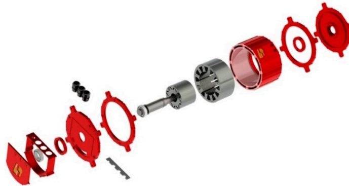
Figure 1. Exploded view of the PMSM to be controlled by the proposed controller.
