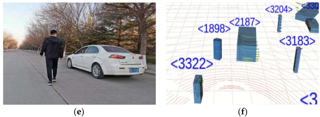
**Figure 7.** Obstacle data-association results. (a) Original scene view at frame 70, (b) frame 70 point cloud data, (c) original scene view of frame 100, (d) frame 100 point cloud data, (e) original scene view of frame 130, (f) frame 130 point cloud data.
