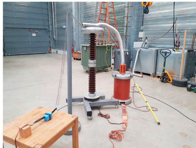
Figure 15. Test of transformer insulating material at 70 kV for 1 min.
