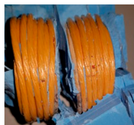
Figure 16. Isolation failure of 2nd test sample.
