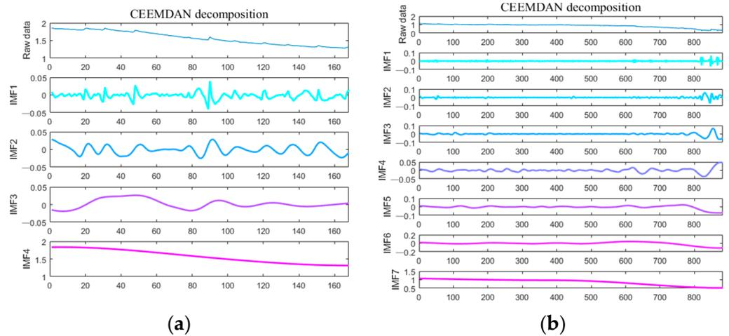
**Figure 9.** CEEMDAN decomposition of battery capacity data. (a) Decomposition of B0005; (b) decomposition of CS2\_35.
