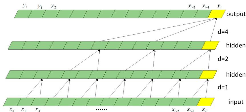
Figure 1. Dilated causal convolutional network architecture of TCN.
