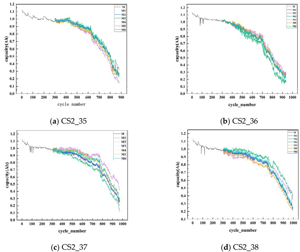
**Figure 14.** Multiple model comparison experiments of CALCE battery (300 predicted starting points). (a) Comparative experiment for battery CS2\_35; (b) comparative experiment for battery CS2\_36; (c) comparative experiment for battery CS2\_37; and (d) comparative experiment for battery CS2\_38.
