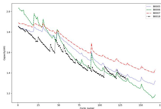
Figure 7. Capacity degradation curves of NASA battery.
