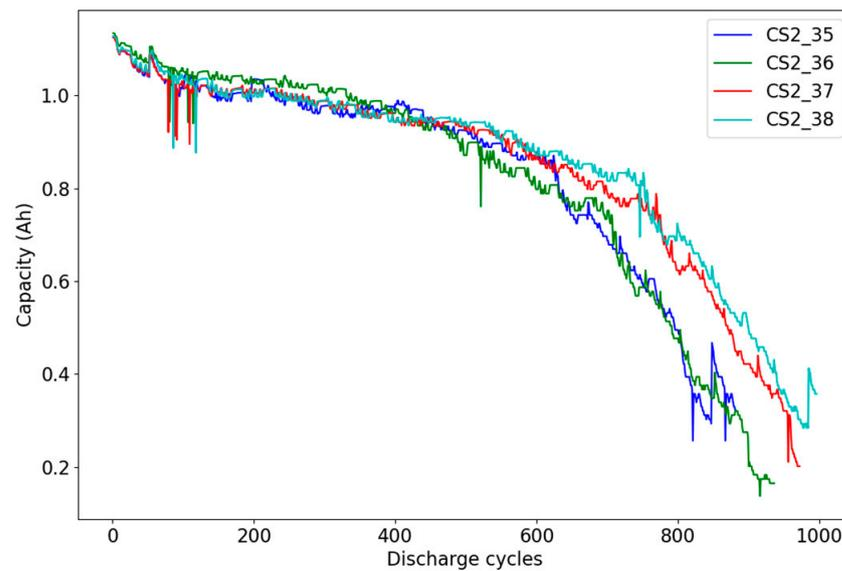
**Figure 8.** Capacity degradation curves of CALCE battery.
