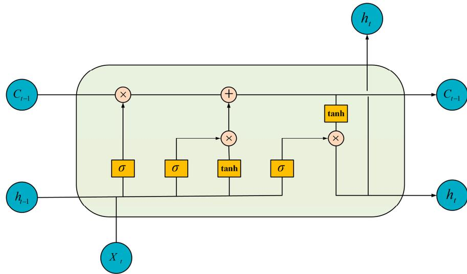
**Figure 2.** Basic structure diagram of LSTM.
