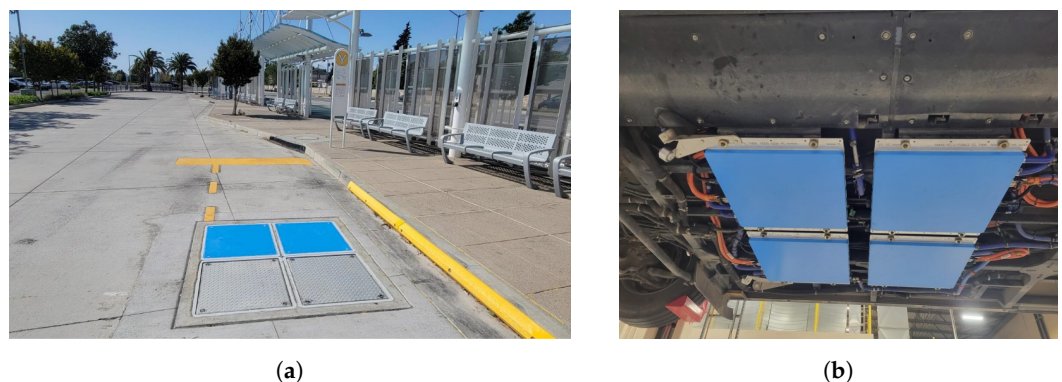
Figure 6. Static wireless charging system developed by InductEV for an electric bus: (a) ground unit (two charging pads) (reproduced with permission from InductEV Inc.). (b) Vehicle unit (four charging pads) (reproduced with permission from InductEV Inc.).
