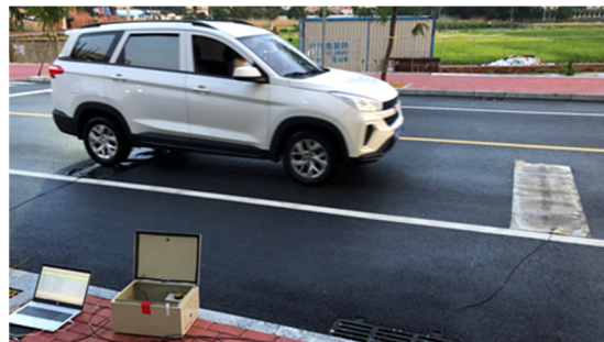
Figure 1. Experimental diagram of axle load signal acquisition.
