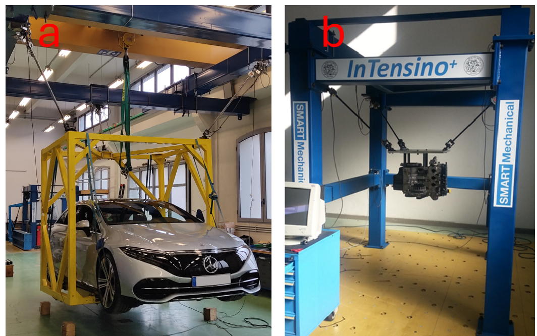
Figure 1. InTenso+ system of Politecnico di Milano. (a) Equipment for full vehicles (max 3500 kg). (b) Equipment for vehicle subsystems (up to 400 kg).
