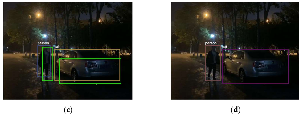
Figure 12. The fusion process in the night scene, where (a) is the actual scene; (b) is the camera detection result; (c) is the result obtained by projecting the 3D detection frame of the point cloud to the image, where the green frame is the 2D projection frame of the point cloud; and (d) is the final fusion result.
