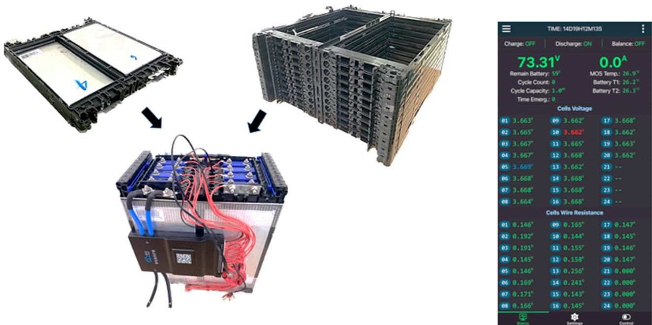
Figure 4. Battery pack and balance with BMS.
