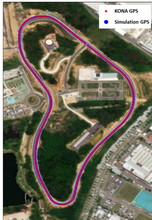
Figure 6. The result of the virtual twin ToD driving test on the expressway. The image represents the actual GPS data of the KONA vehicle (red line) and the GPS data obtained from the simulator (blue line) overlain on the satellite imagery of the C-track.
