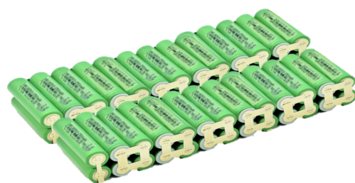
Figure 2. Internal configuration 18,650 battery pack. Source: Author's own elaboration.
