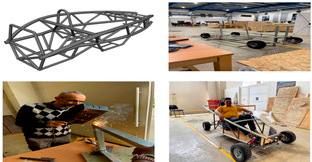
Figure 5. Chassis construction progress.
