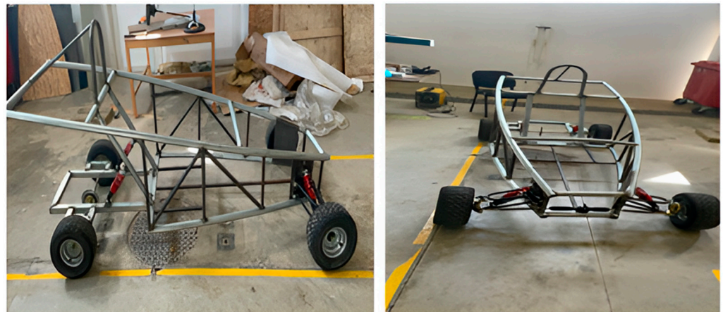
Figure 11. Wheel mounting on the chassis.
