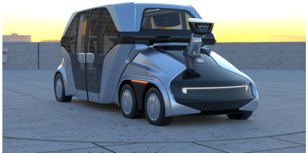
Figure 1. The EDAG CityBot connected, automated, shared and electric (CASE) vehicle equipped with a people mover trailer module. Copyright 2023 EDAG Group.
