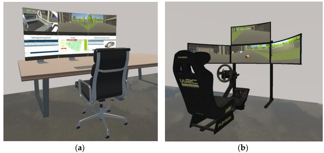
Figure 4. The operation center consists of a workstation for the (a) dispatcher and the (b) teleoperator.
