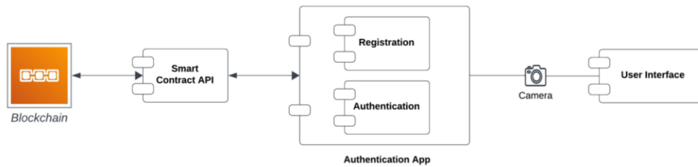
Figure 3. UML component diagram of registration and authentication model.
