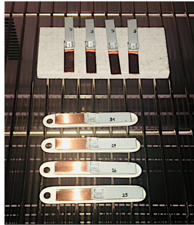
Figure 4. Samples in the furnace for accelerated aging.
