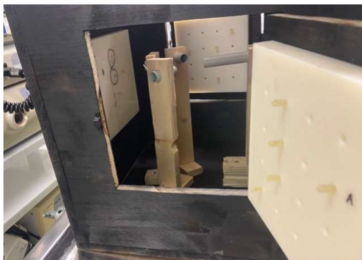
Figure 6. Training box from the lateral view through the side door. On the door is a fitted platform with pins used to exercise movements. Through the door, a set of tubes and other platforms with different tasks are visible.
