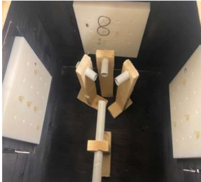
Figure 4. Ground view inside the training box. Visible is the set of tubes that lead to different platforms with different tasks.
