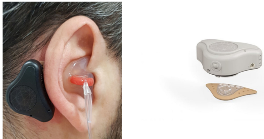
Figure 1. Right ear. ABCD device in place in a typical subject, where the ear canal is occluded by a custom silicone plug. On the right, a commercial figure of the ABCD showing the external laterale surface is visible, and the microphone ports are visible on the right (in the lower part of the device when worn on the right side).
