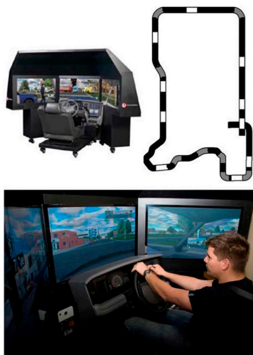
Figure 1. MPRI PatrolSim IV driving training simulator (top left), structure of the 28-mile road course with measured straights in white and measured curves in gray (top right), and a demonstration of driving the simulator in a suburban scenario rather than the rural highway scenario used in these experiments.
