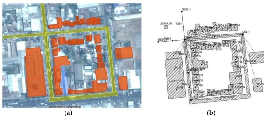
Figure 3. (a) Surface of green roofs (orange areas) and collectors (yellow areas) in Case Study 1; and (b) Hydrological model in SWMM.
