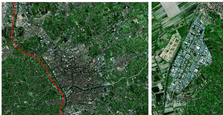
Figure 5. Barrier effect (dotted line in red) of A-30 highway preventing urban sprawl growth to the East ( left ) and industrial estate developed together with MU-31 road ( right ).
