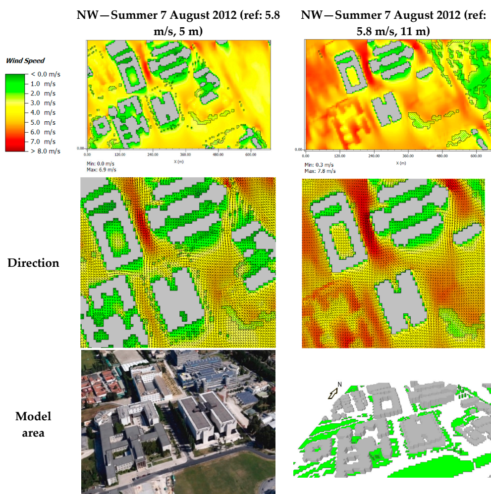
Figure 8. ENVI-met micrometeorological simulation of average wind conditions during summer at 5 m and 11 m, at 5 p.m., around the Arquivo Nacional da Torre do Tombo (“H” shaped building in the center). The trees are represented by the green spots around that building (picture top left). The trees could not be implemented exactly. The direction of deformation of the trees (black arrows) are shown in the middle of the figure. The model area is presented at the bottom.
