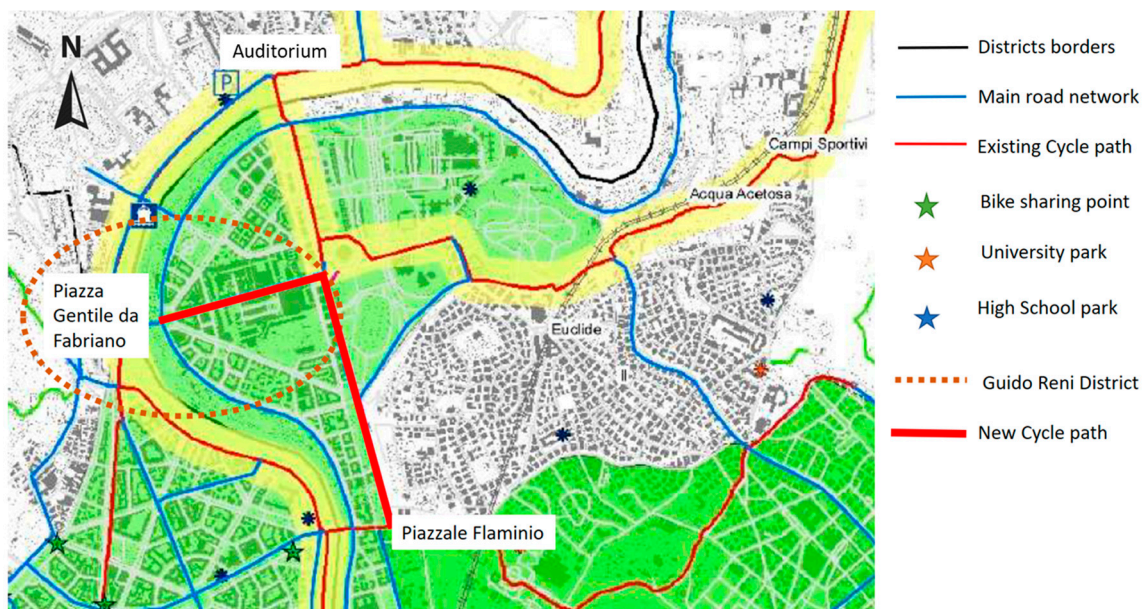
Figure 1. Existing layout of the functional transport network.
