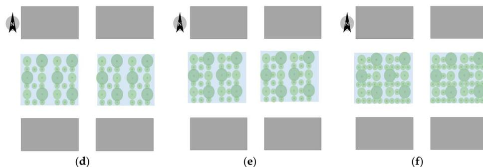
**Figure 4.** Models of plant collocations under different ratios of trees to shrubs. (a–c) were middle- and low-level plant collocations corresponding to tree to shrub ratios of 2:3, 1:2, and 1:3; (d–f) were middle- and high-level plant collocations corresponding to tree to shrub ratios of 2:3, 1:2, and 1:3. Each greening configuration corresponded to a kind of underground space overburden thickness that could meet the requirements of growth for plants (picture source: ENVI-met).
