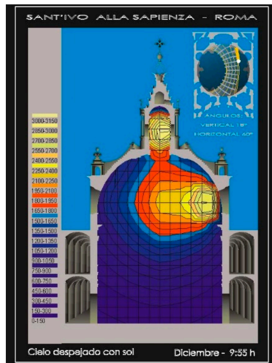
Figure 23. Simulations at Sant'Ivo by Borromini in Rome. December at 9:55 am. Clear sky plus sun. Source: Almodovar-Melendo.
