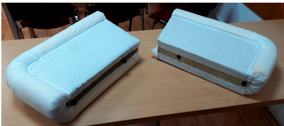
Figure 8. Sofa side with comfort a layer from composite (left), from wood (right).
