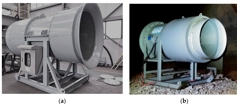
Figure 2. Two fans developed for the pressurization ventilation experiments: (a) 37 kW high-pressure fan; (b) 15 kW low-pressure fan.
