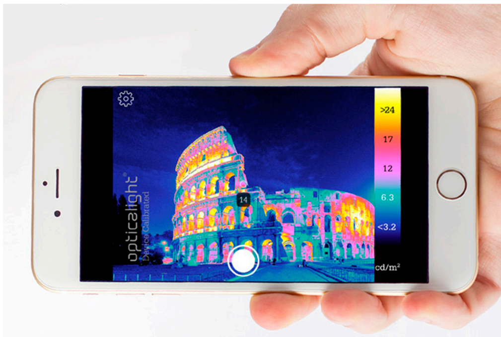
Figure 5. An example of the results from a typical outdoor luminance measurement in \text{cd}/\text{m}^2 taken by a video luminance meter mobile phone application with a false color image function for easy evaluation. False color assigns different colors to areas of different luminance exposure in the image. Source: Opticalight's figure.
