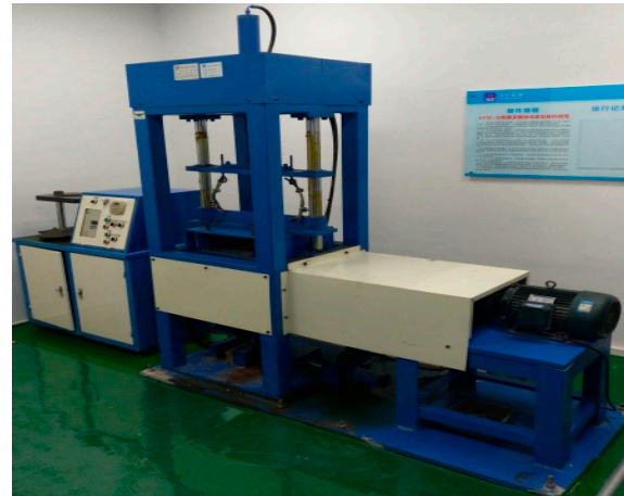
Figure 1. Vertical vibration testing equipment (VVTE) schematic.
