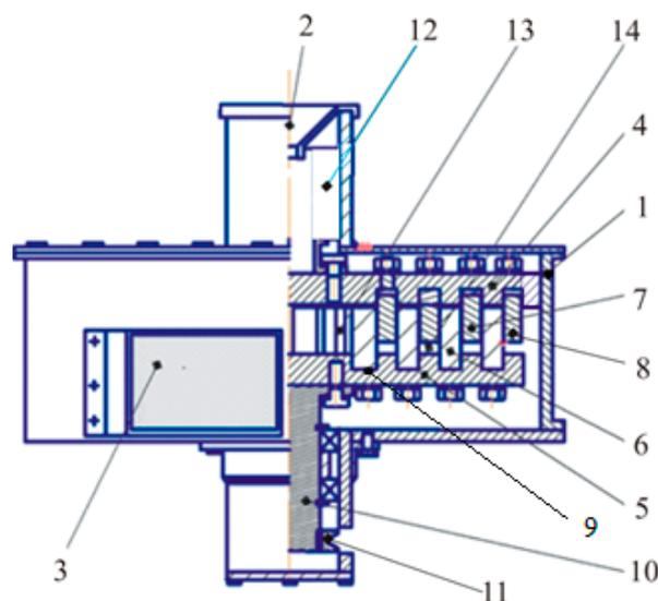
**Figure 1.** Design overview of a rotary-centrifugal device for grinding bulk materials. Parts include: 1—case; 2—loading (input); 3—output nozzles; 4—upper disk; 5—lower movable disk; 6—annular protrusions; 7—knives; 8—outer row of knives; 9—groove; 10—drive shaft; 11—pulley; 12—receiving chamber; 13—radial windows; and 14—working chamber.
