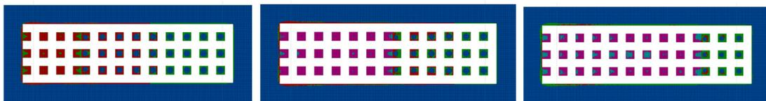
(a) Plastic zone development of the stope where the compressive strength of the backfilled pillars was 1 MPa and the recovery distances were 54, 108, and 162 m.
