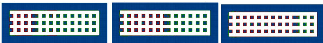
(b) Plastic zone development of the stope where the compressive strength of the backfilled pillars was 2 MPa and the recovery distances were 54, 108, and 162 m.
