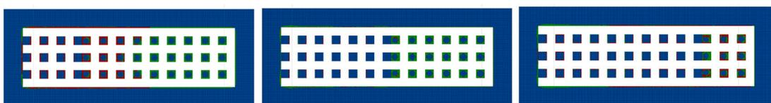
(c) Plastic zone development of the stope where the compressive strength of the backfilled pillars was 3 MPa and the recovery distances were 54, 108, and 162 m.
