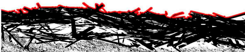
Figure 7. Measurement of the residual cover thickness (RCT) by using MATLAB: (a) photo of the measured area of straw; (b) using Matlab to process the photo and get the RCT.
