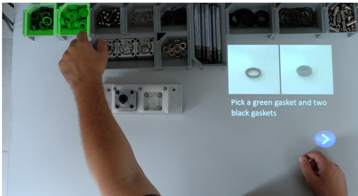
Figure 6. Projection-based assistance systems (Ulixes “Der Assistent”) to guide people with disabilities through a complex assembly cycle (picture taken in Smart Mini Factory – Laboratory for Industry 4.0, Free University of Bozen-Bolzano).
