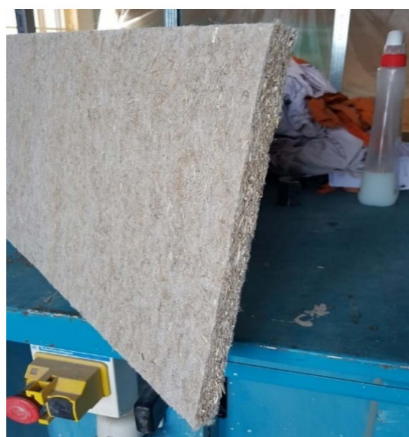
Figure 2. Reinforced hemp insulation panel used in the project.
