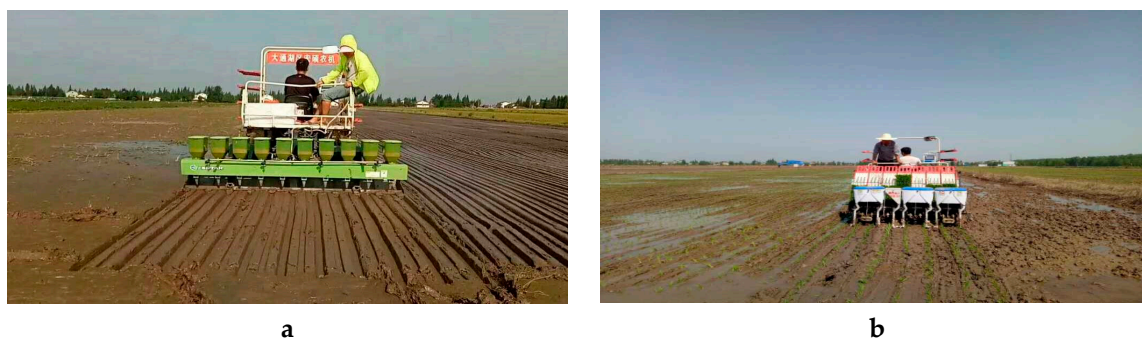
Figure 3. (a) Direct rice seeding using 2BDCSP Precision Rice Hill-Drop Drilling Machine; (b) mechanical transplanting using YANMAR VP7D25 Rice Transplanter.
