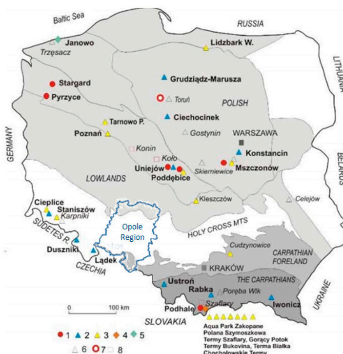
Figure 1. Geothermal installations in Poland, 2017: 1-district heating plants, 2-health resorts, 3-recreation centers, 4-wood drying, 5-fish farming, 6-recreation centers in realization, 7-heating system at early stage, 8-some expected co-generation installations. Source: Kępińska 2019.
