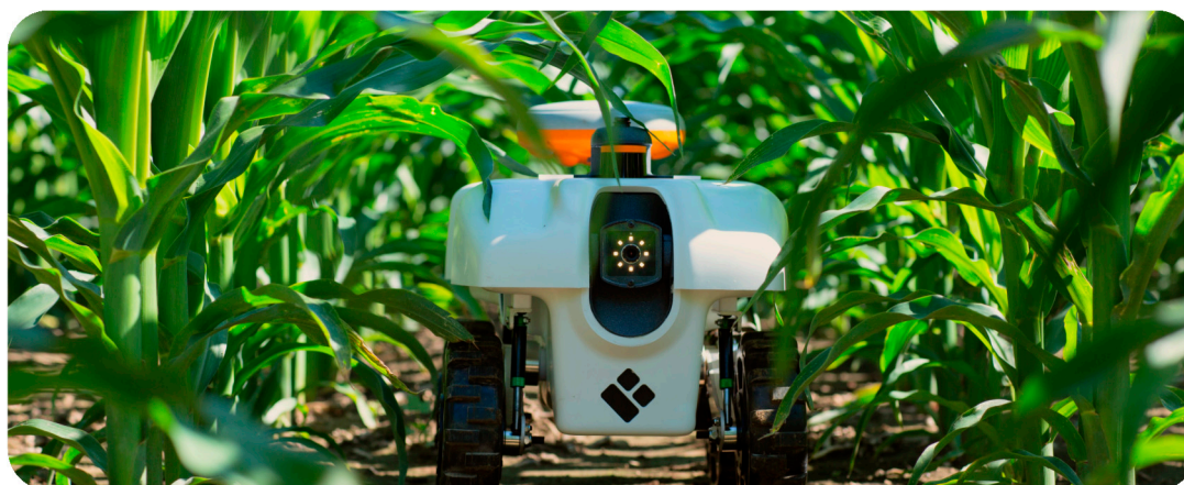
Figure 7. The TerraSentia robot is compact enough to fit between the rows of corn. The 2019 model manufactured by EarthSense ( www.earthsense.co ) is 31.75 cm (12.5 inches) wide, 54.1 cm (21.3 inches) long, and 35.56 cm (14 inches) tall and weighs around 13.6 kg (30 lbs). About 40 robots were made in 2019 and deployed across fields in the US. Users reported a battery life of between 4 and 6 h.
