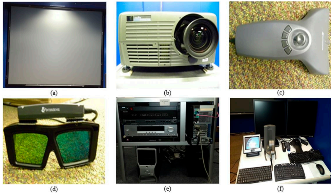
Figure 7. Hardware used: (a) screen; (b) rear projector; (c) hand wand; (d) shutter glasses with head tracker; (e) virtual reality (VR) hardware controller with workstations; (f) AMX controller with space mouse and space ball.
