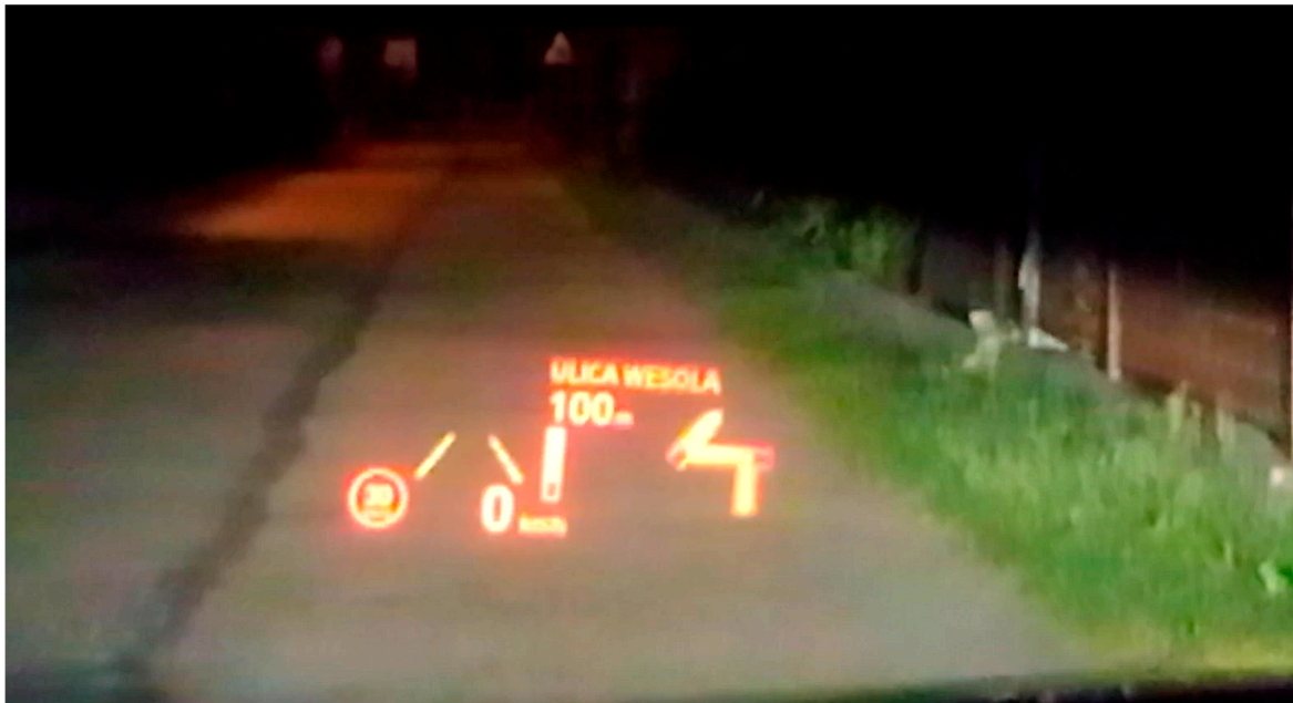
Figure 3. Car navigation whose map is displayed digitally on the windshield. Resource: Own elaboration.
