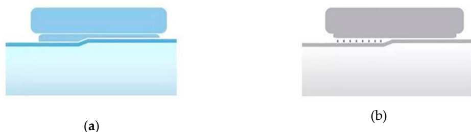
Figure 4. Comparison between floating and ordinary wipes: (a) Floating wipe with fit elastic; (b) ordinary wipe with a suspended gap.
