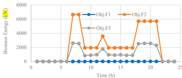
**Figure 16.** Biomass Energy (Pwb) Scheduling in Configuration 3.
