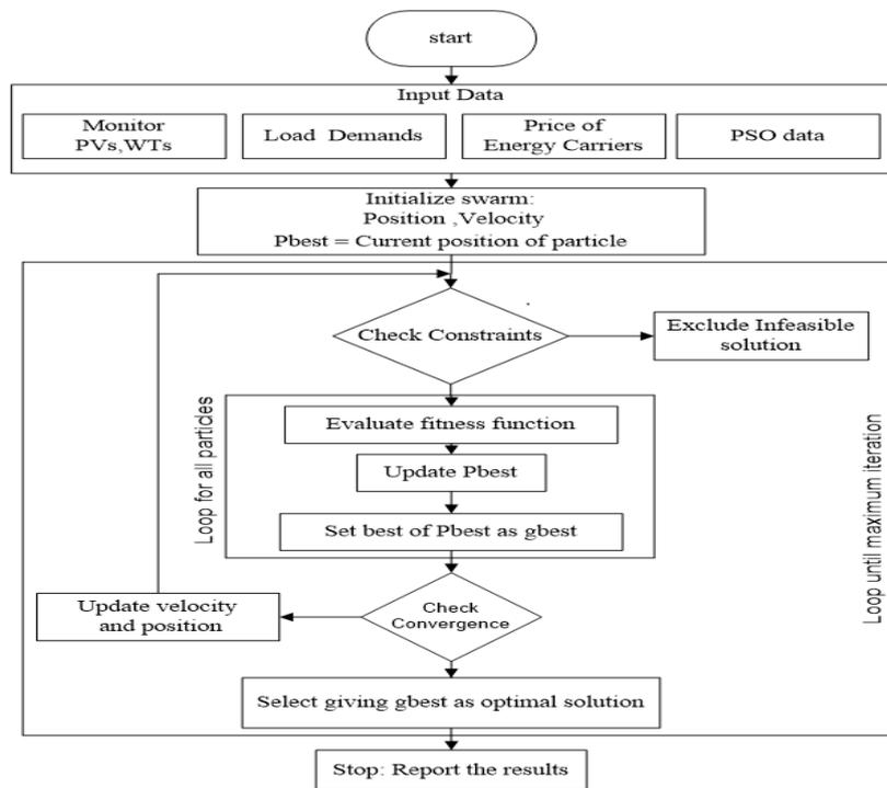
Figure 3. Flowchart of particle swarm optimization (PSO) based Scheduling Algorithm.
