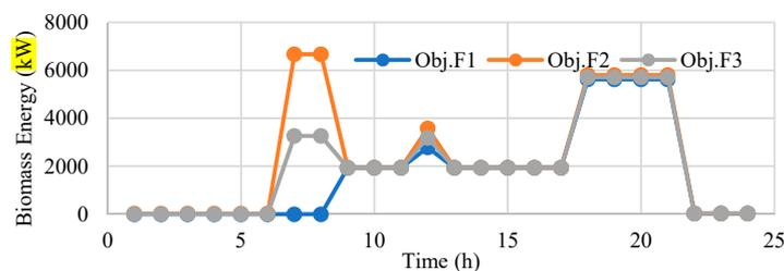
Figure 11. Biomass Energy (Pwb) Scheduling in Configuration 2.
