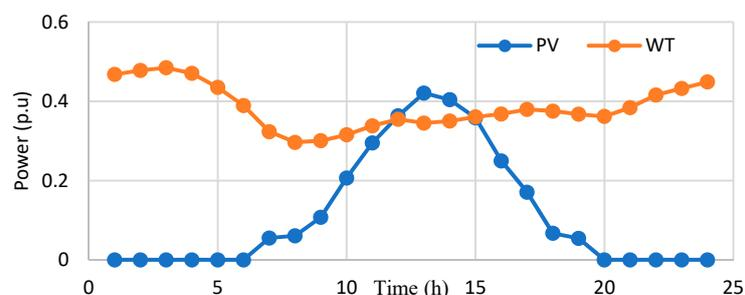
Figure 6. Output Power from PV and WT.
