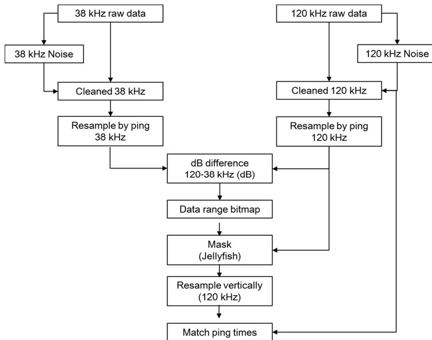
Figure 2. Data processing flowchart to identify *N. nomurai* using frequencies 38 and 120 kHz.
