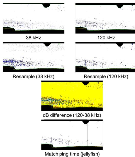
Figure 3. Echogram example of data processing flowchart to identify the echo signals of *N. nomurai* using frequencies 38 and 120 kHz.
