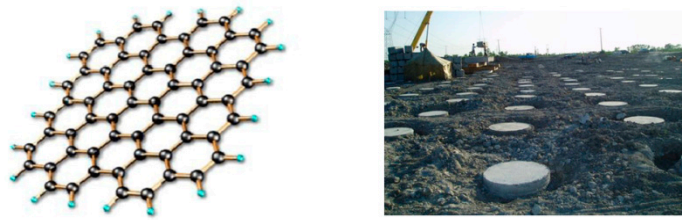
(a) Analogy of phononic crystal and piles with a periodic arrangement.
