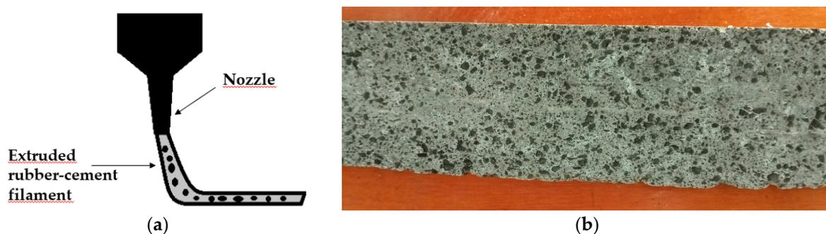
**Figure 14.** Schematic illustration of the deposition process of printable rubber-cement mixes (a). The internal section of P-G50/50 slab (b).
