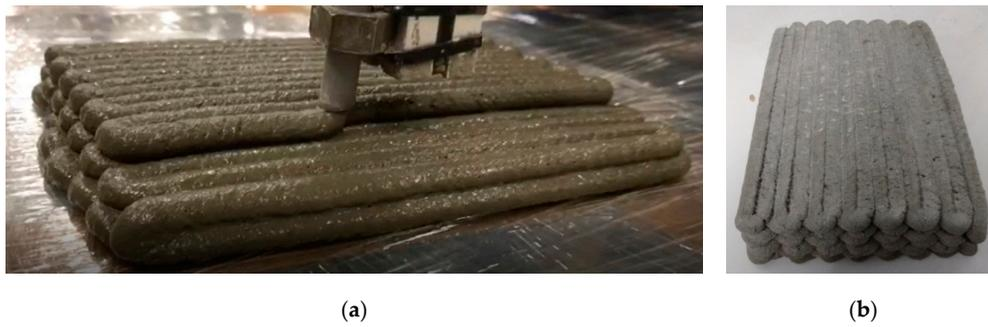
**Figure 2.** Extrusion of fresh material (P100 mix) during the printability test (a) and six-layer 3D printed slab in hardened state (b).
