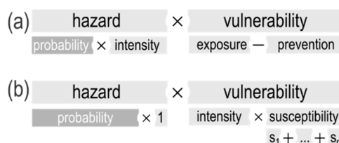
Figure 1. Risk components of (a) generic concept and (b) vulnerability concept by [33]. Note that damage intensity as a subcomponent shifts between both concepts. s_1 \dots s_n : susceptibility components. Probability is highlighted, as it turned out to be the most variable and least defined component in the framework.
