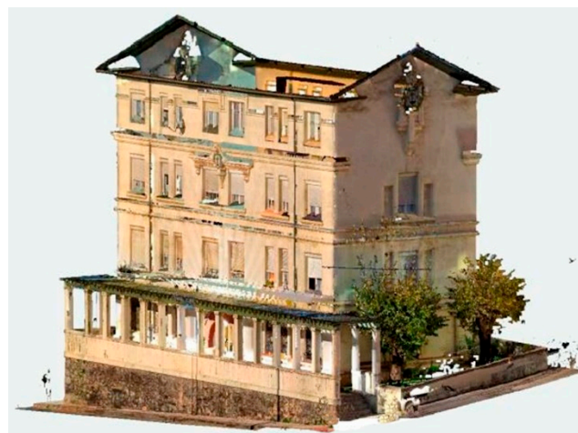
Figure 8. 3D Model produced by the laser scan (Source: Urquizo&NorthBIM).
