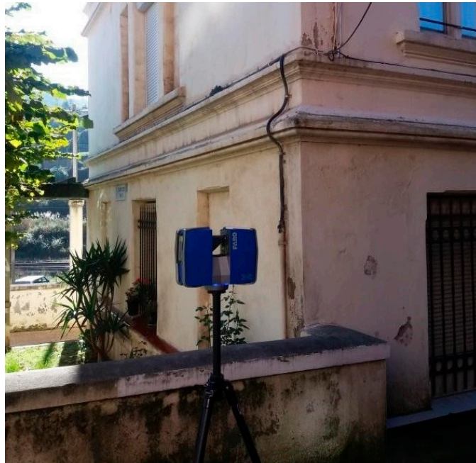
Figure 6. FARO Focus 3D×330 scanner on a tripod (Source: Urquizo Ingenieros&NorthBIM).
