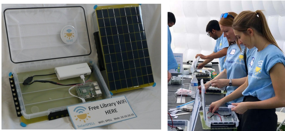
Figure 1. Assembling the SolarSPELL libraries, and the finished product: a SolarSPELL library.
